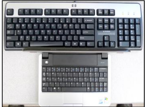
The Dell Mini 9's keyboard is tiny compared to a full-sized desktop keyboard.
