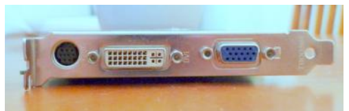
Even inexpensive graphics cards frequently offer two monitor connections. This graphics card supports two monitors, offering a DVI (white) and a VGA (blue) connector.
