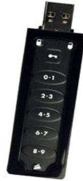
Corsair's Flash Padlock uses a novel type of physical data security.
