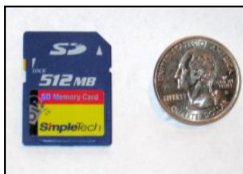
Figure 1: This memory card, the size of a U.S. Quarter, can hold over 200 digital pictures from a megapixel (6MP) digital camera.
