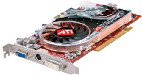
Figure 3: This graphics card has both analog (blue connection on left) and digital (white connection on right) outputs.
