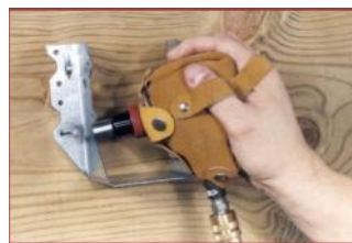
Pneumatic palm nailers allow you to quickly drive nails in awkward locations.
