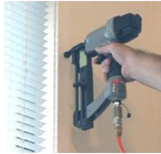
An air-powered stapler attaches molding in a jiffy.
