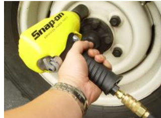
Pneumatic impact wrenches can break free stubborn lug nuts.
