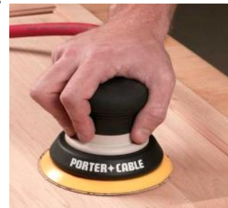
An air-powered sander preps wood for finishing.
